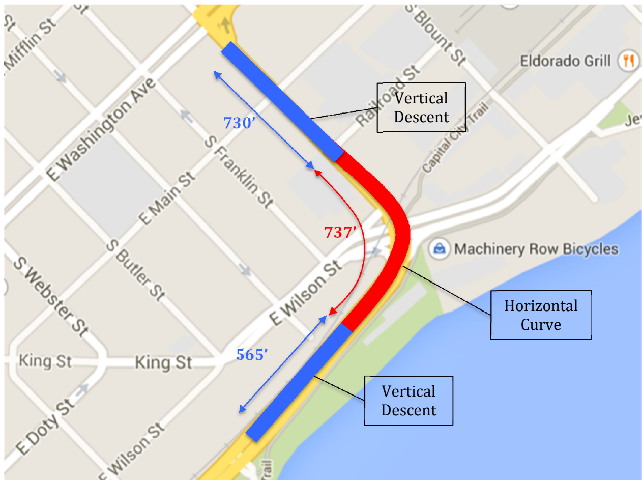
Figure 5: Tunnel Plan View
